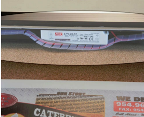
Ballast/Transformer concealed inside Display Case
